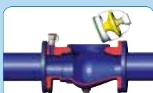
Remove the whole spring, closing system and seal.
